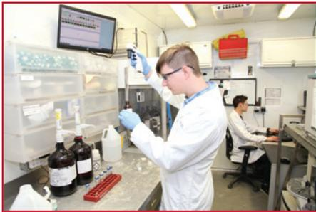
Each mobile laboratory is equipped with 2 Gas Chromatographs (GC) allowing for simultaneous F2-F4 and BTEX/VH analysis.
